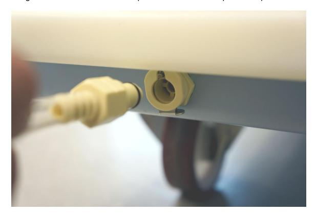
6. Disconnect the drain hose by pressing the silver button to release.
