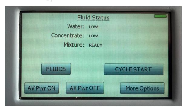
8. The concentrate status will show the level in the concentrate reservoir. If the level is LOW or EMPTY, Press the "Concentrate Load" button.
