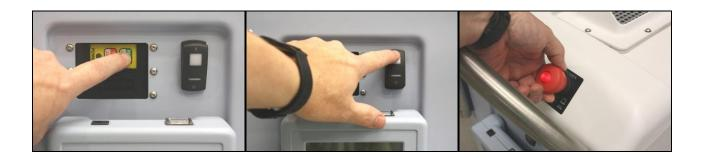
4. Turn the remote control on by pressing the power switch on the top of the remote.
