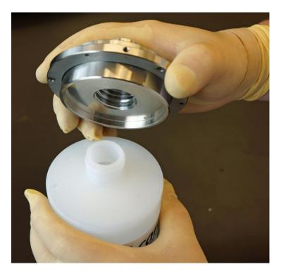
3. While holding the bottom of the bottle, screw the adapter onto the bottle in a clockwise direction.
