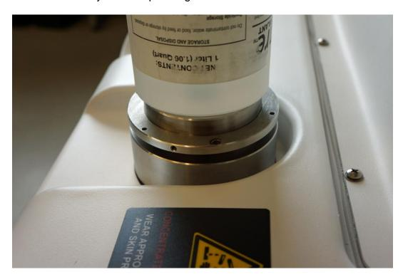
6. Immediately push the bottle down completely and firmly. There should be no gap between the adapter and receiver on the machine.
