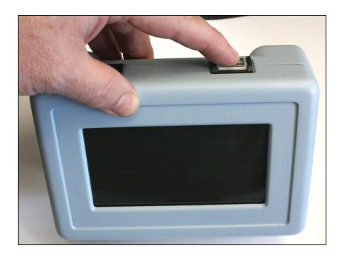
5. Upon power up, the display will show a welcome screen with the company logo. In the upper-right corner of the display is a battery status indicator. This indicator shows the state of the internal rechargeable batteries. When the indicator gets low or starts blinking, charge the batteries by hanging the remote on the machine under the handle, or connect it to the wall charger.
