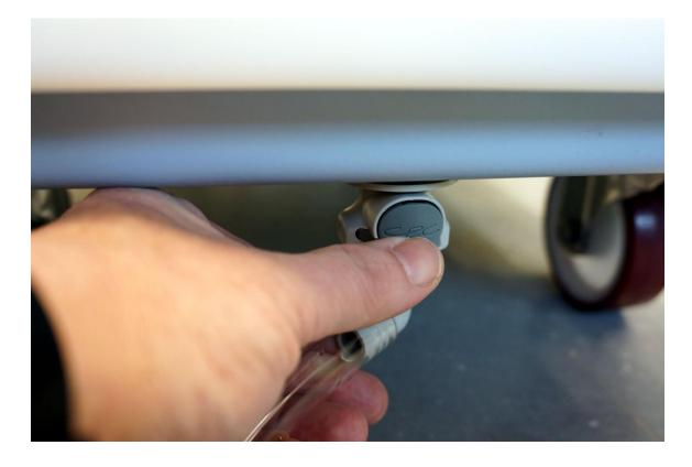
5. Over time, the main blower can accumulate fluids (a swishing sound can be heard during deploy), connect the smaller hose to the connector on the back of the machine (handle end) and route it to a drain. Draining the main blower does **not** require the machine to be powered up.
