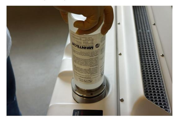
5. Turn the bottle assembly until the pins align.
